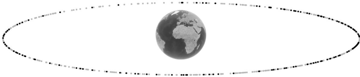
**Figure 1:** The geostationary belt. As of January 1, 2020, the U.S. Space Command's Combined Space Operations Center (CSpOC) database contains the orbital elements for nearly 800 satellites in GEO. The black points represent satellites launched within the past five years. *Data Source: U.S. Space Command Combined Space Operations Center / Space-Track.org.*
